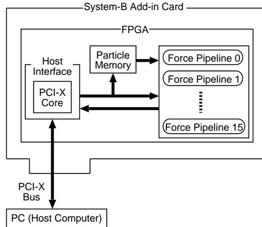
Figure 2: Block diagram of System-B.
