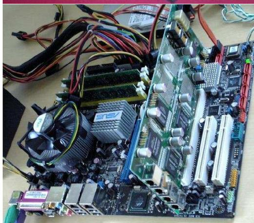
Figure 3: Photograph of the add-in card for System-A (PLDA PXPDKSXGX40, top), and System-B (KFCR GRAPE-7, bottom).
