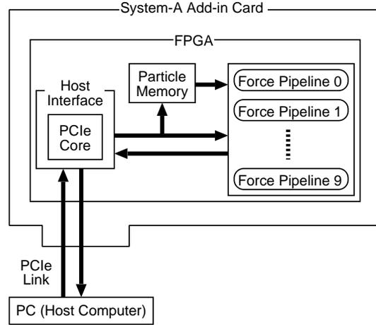
Figure 1: Block diagram of System-A.
