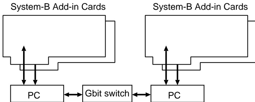
Figure 6: A small parallel system.
