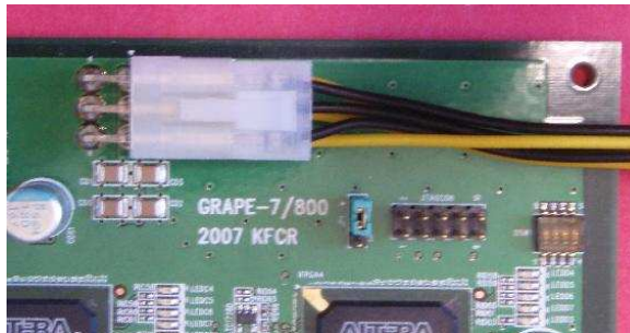
Figure 9: Power cable connection (Model 800).
